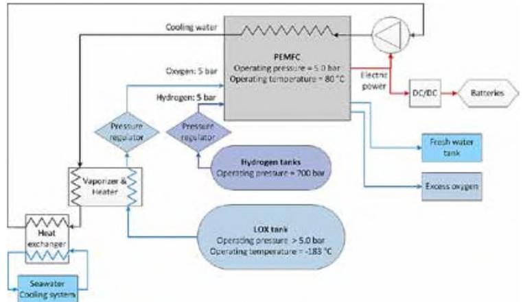
Figure 4. Overview of complete fuel cell system.
