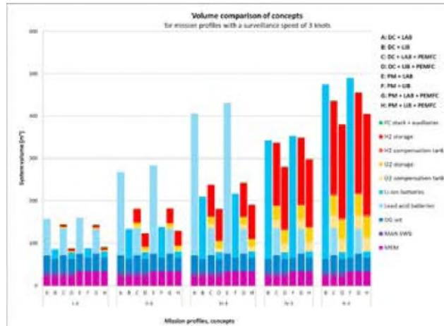
Figure 7. Example of results: Volume of components for all concepts for missions with three knots surveillance speed.
