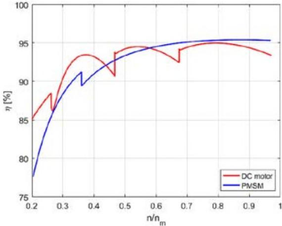
Figure 6. Modelled efficiency curve of the DC compound motor and the PMSM motor.
