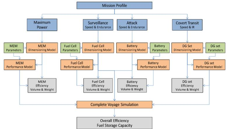
results in the required battery dimensions and mass. The corresponding diesel generator power is calculated from the defined in-discretion ratio (IR) for the covert transit phase. The IR is defined as:
