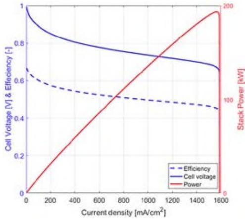
Figure 3. Polarisation curve of a single PEMFC.
